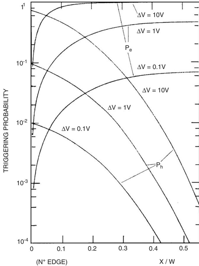
Fig. 14. Triggering probability for different positions of carrier generation (see text).
