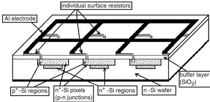
Fig. 6. Basic structure of a Geiger-mode avalanche photodiode. Taken from Sadygov [12].
