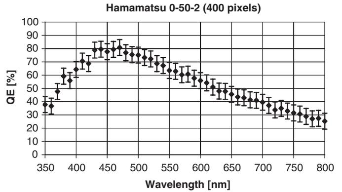
Fig. 12. Quantum efficiency as function of the wavelength.
