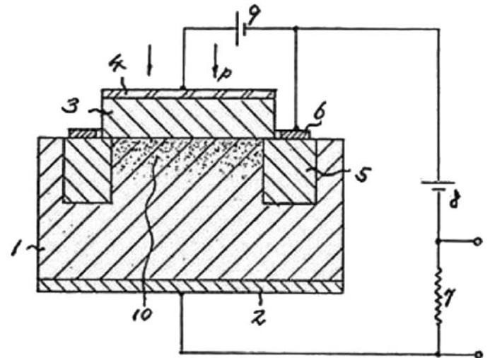
Fig. 3. Structure of the detector developed in Japan.
