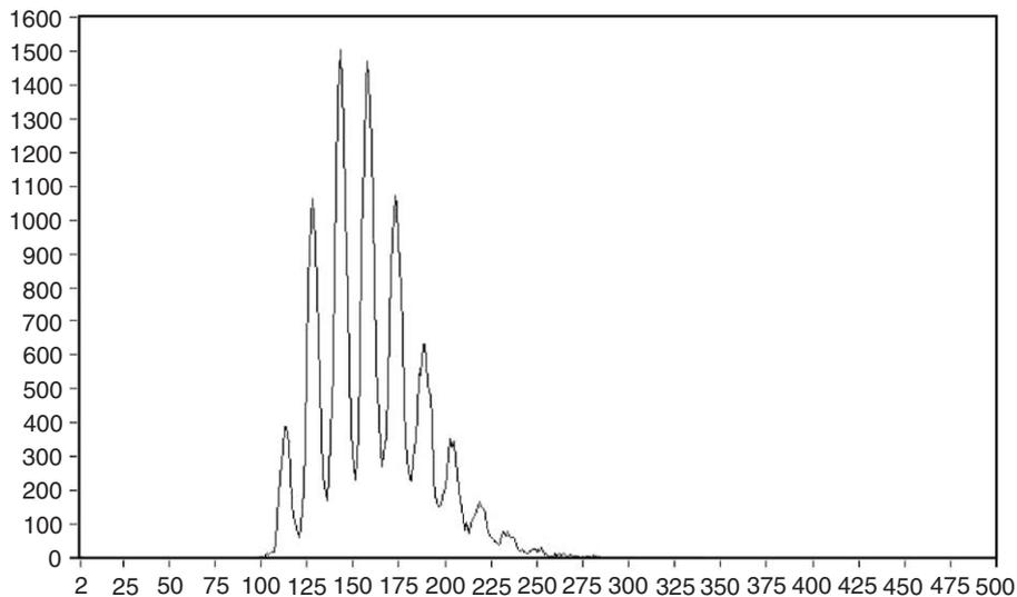
Fig. 7. Oscilloscope picture of the signal from a G-APD (Hamamatsu 1-53-1A-1) recorded without amplifier (a) and the corresponding pulse height spectrum (b).
