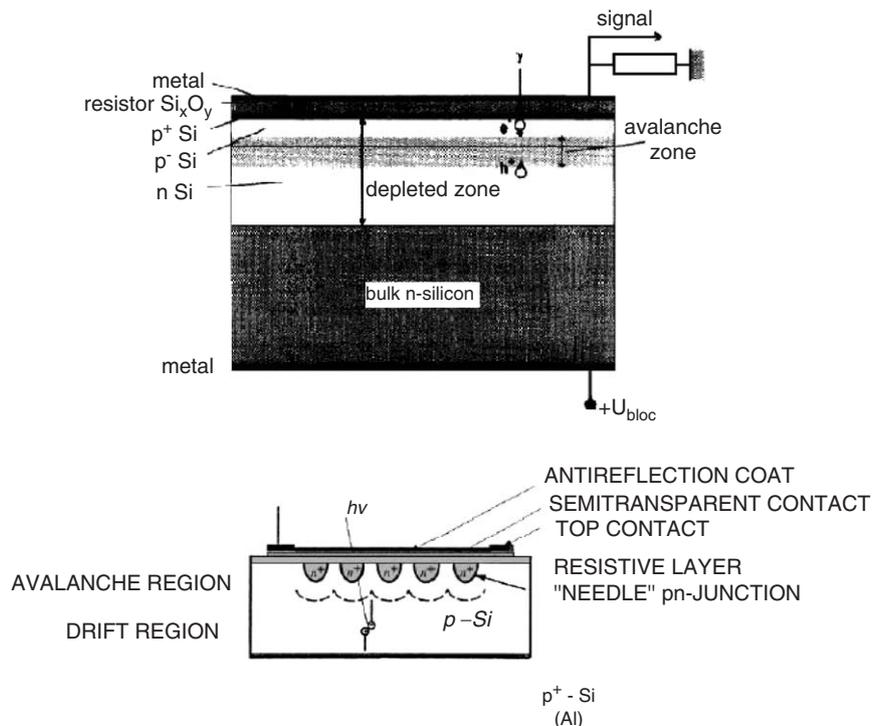
Fig. 5. Examples of MRS APDs structures. The picture on top is taken from Antich et al. [9] and the picture at the bottom is from Saveliev and Golovin [10].
