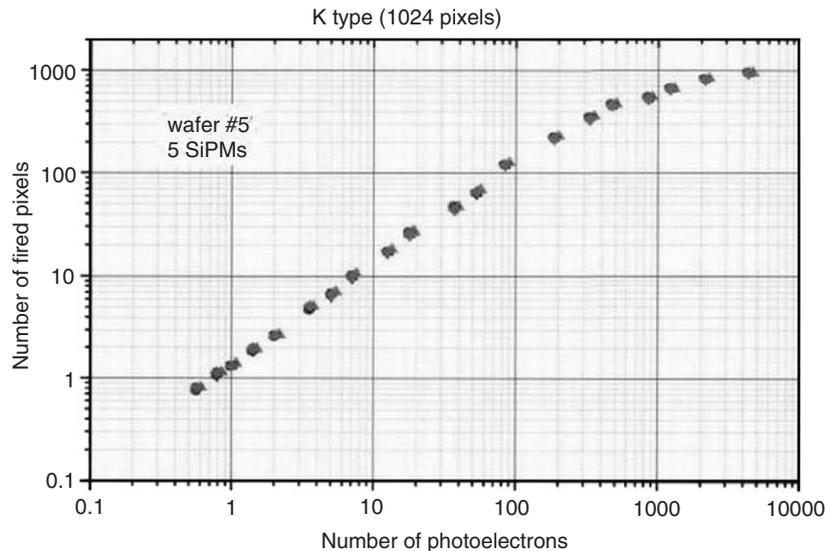
Fig. 8. The number of fired cells which is proportional to the signal amplitude as function of the primary photoelectrons. From Andreev et al. [14].
