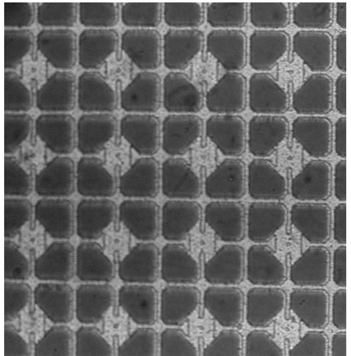
Fig. 13. Microscopic view of a G-APD produced at JINR in Dubna, Russia.
