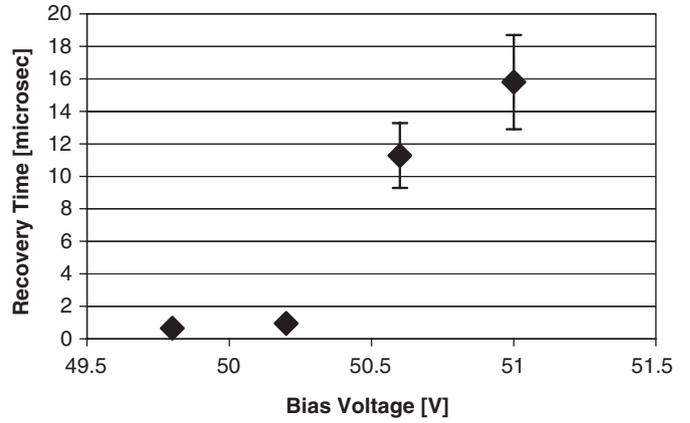
Fig. 15. Recovery time for 4 different settings of the bias voltage.
