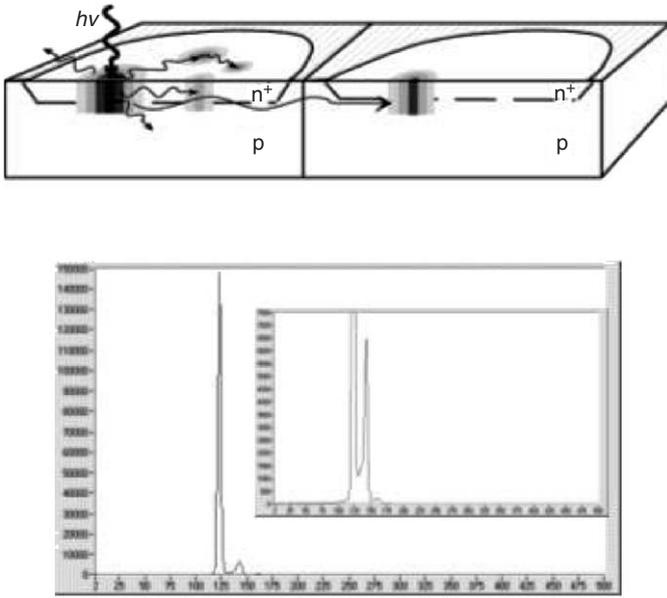
Fig. 10. Optical crosstalk in a G-APD (top) and a pulse height spectrum of events triggered by one single carrier (bottom). Events where a second and even a third cell was fired are visible as satellite peaks. The insert is the same histogram but with the vertical scale is reduced by a factor of 20.
