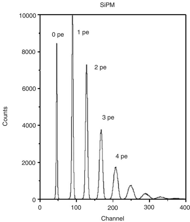
Fig. 1. Pulse height spectrum of light pulses with very low intensity recorded with a G-APD. Taken from Buzham et al. [2].
