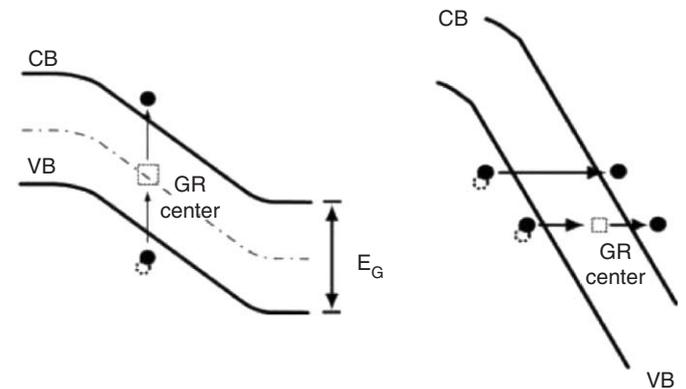
Fig. 9. Thermally (left) and field-assisted generation (right) of free carriers which can trigger a breakdown.
