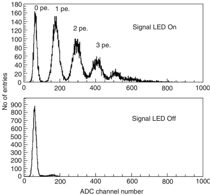
Fig. 4. Pulse height spectrum of light pulses with very low intensity recorded with a VLPC. Taken from Bross et al. [8].
